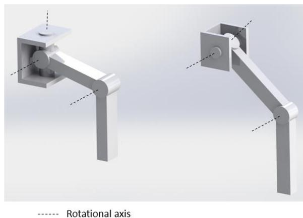
*Figure 3:* The left figure is a model of an insect-type leg configuration. The right figure is a model of mammal leg configuration.
