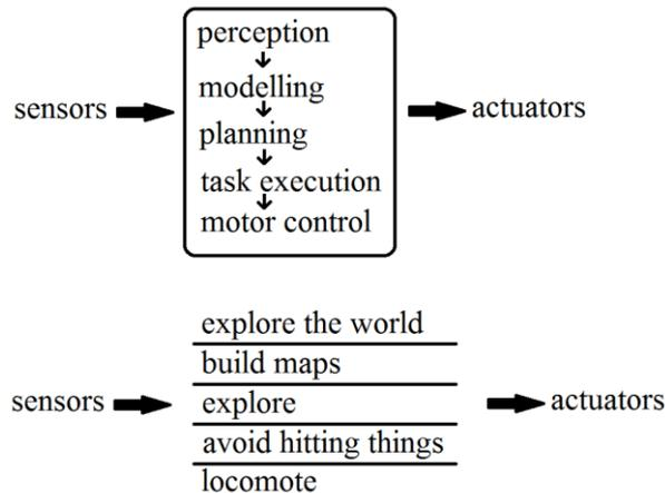
*Figure 2:* The principle of traditional AI is explained. The sensory information is required to penetrate into every single layer before a decision can be made. Therefore, it is time consuming and not applicable to highly dynamic world. Conversely, SA as shown in the lower figure decomposes the behaviour into layers with various priorities (Brooks, 1991)
