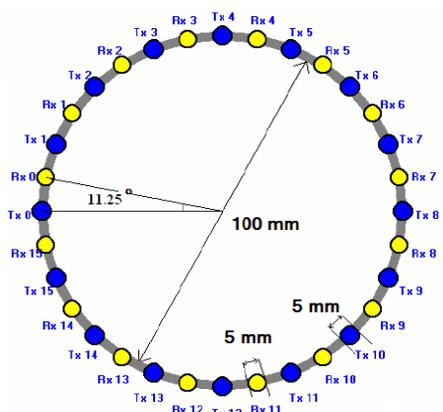
Figure 1 Sensors configuration for optical tomography system [6]
